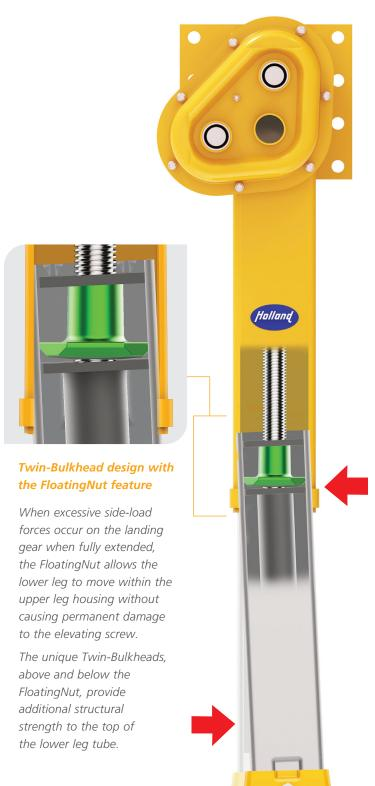
Cranking a landing gear with a bent elevating screw can be an extremely unpleasant experience. Unlike competitive landing gear, the ATLAS has an exclusive special feature to prevent a bent elevating screw from happening.
